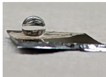
DI water on vertically aligned nanowires
